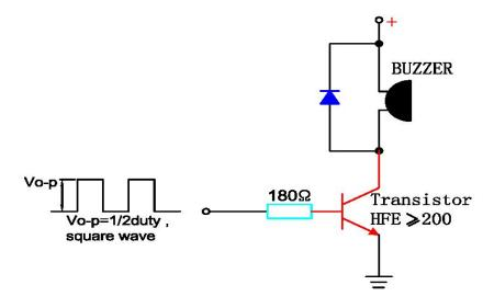
The base current Ib should high enough so that it saturates the collector current of the transistor with the CB load.
