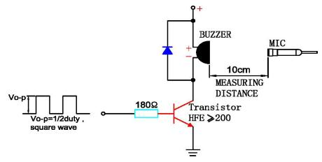
In the measuring test, buzzer is placed as follows:
