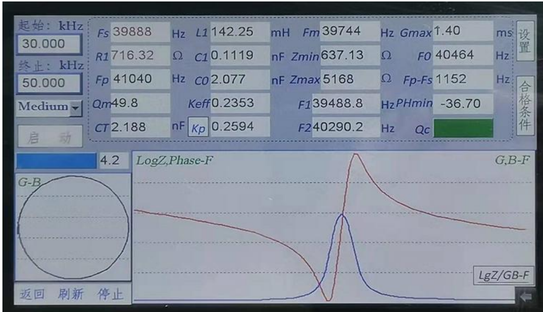
频率-阻抗特性曲线图/Freq-R1.characteristics
